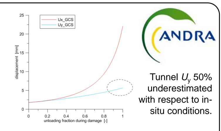
> Further upgrades must include elastic anisotropy (  $E_x = E_z > E_y$  ) and <u>hardening+softening behavior</u>.
